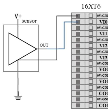
Figure 8-29 Analog voltage input connect to sensor
