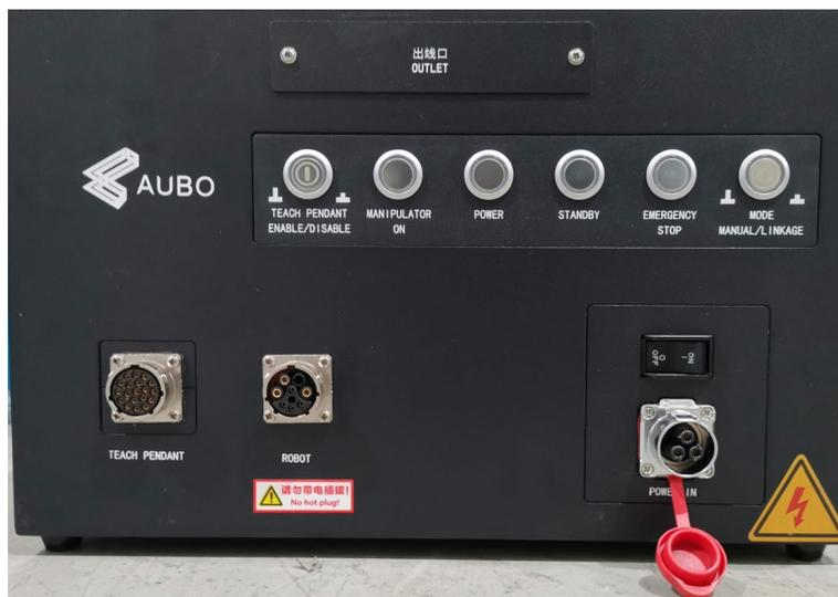
Figure 7-2 Front panel of the control box
