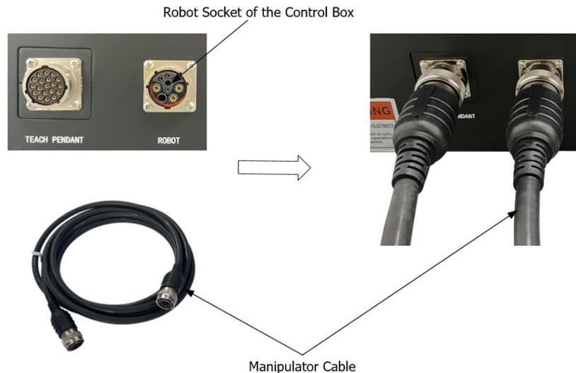
Figure 6-10 Manipulator cable connected to the control box
