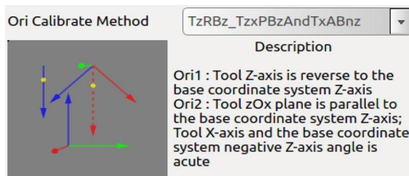
Figure 10-35 TzRBz\_TzxPBzAndTxABnz type calibration method
