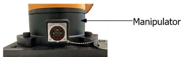
Figure 6-11 Manipulator cable connected to the Manipulator
