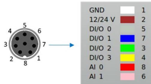
Figure 8-36 Robot Tool I/O wiring order
