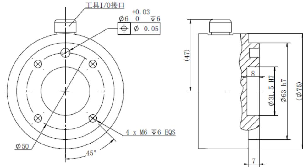
Figure 6-8 Mechanical dimensions of end-effector flange, unit: mm.
