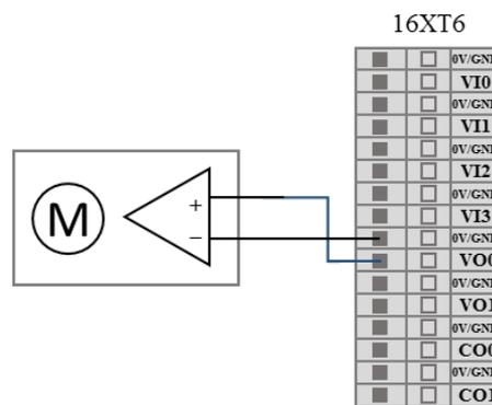
Figure 8-30 Analog voltage output connect drive device
