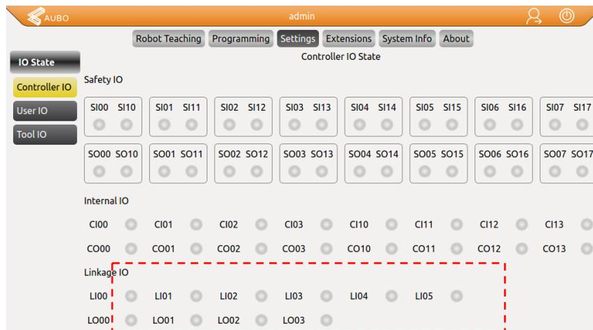
Figure 7-10 AUBOPE software "Settings" tag, Linkage IO status
