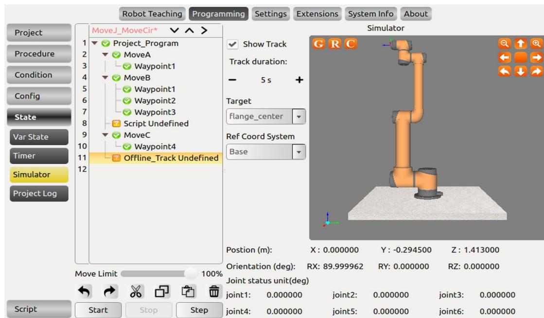
Figure 11-74 Simulation model
