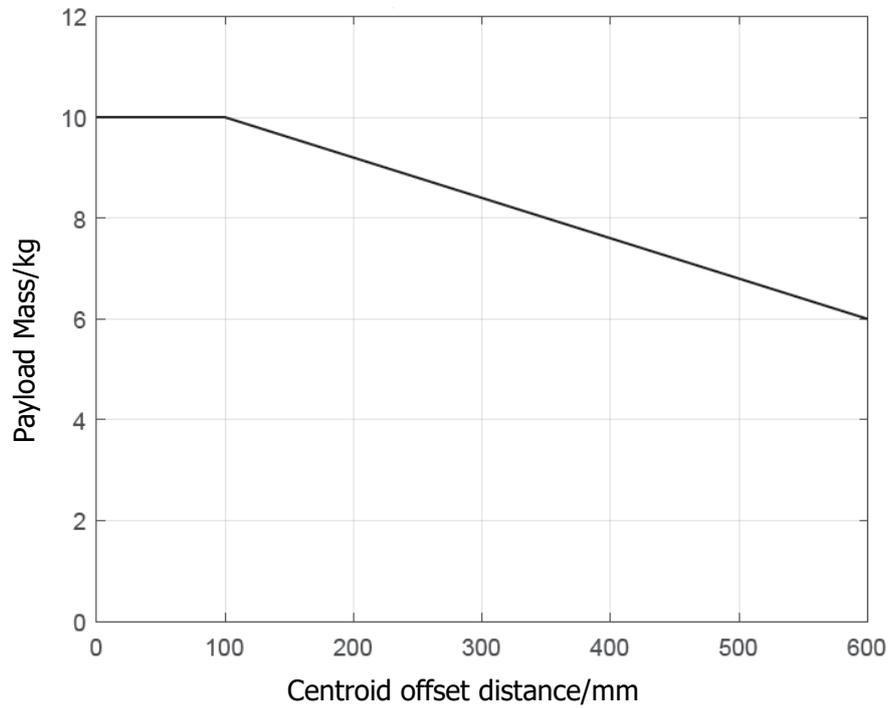
Payload centroid range has shown above, in which x-axis represent the center of gravity offset which is the distance between end-effector flange focus and tool focus.
