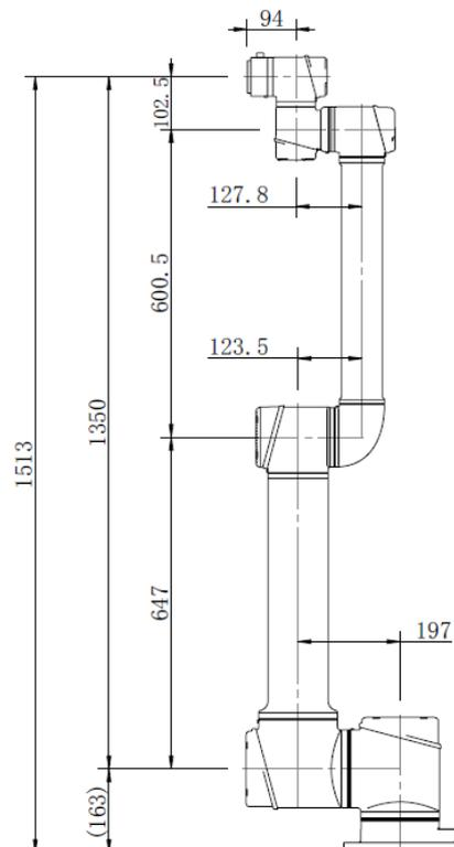
Figure 6-1 AUBO – i10 mechanical dimensions, unit: mm
