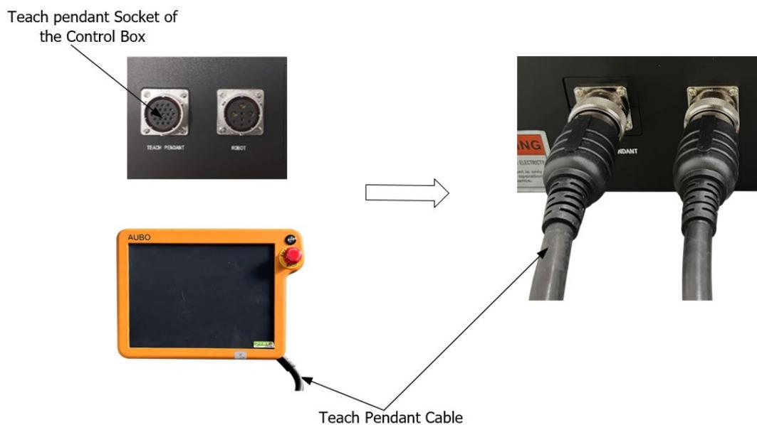
Figure 6-9 Teach pendant cable connected to control box
