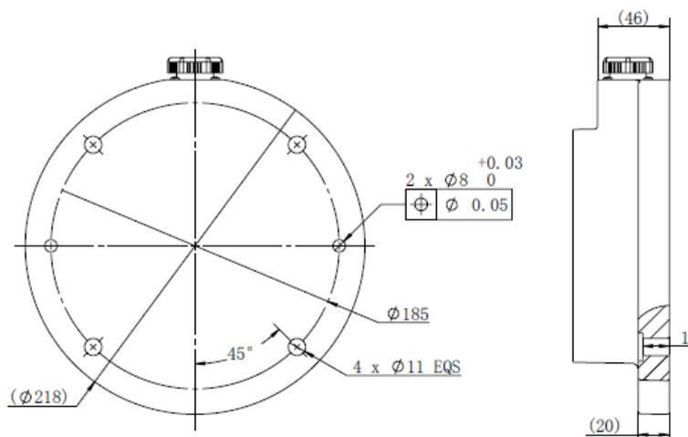
Figure 6-6 : Mounting whole size of the manipulator base.
