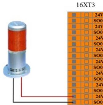
Figure 8-23 AUBOPE operation indication output connection mode
