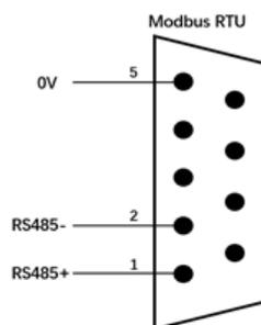
Figure 8-1 Modbus pin description
