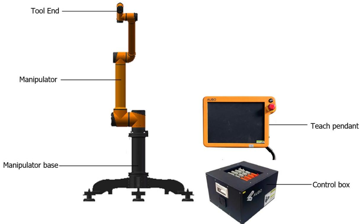
Figure 5-1 AUBO – i10 robot system
