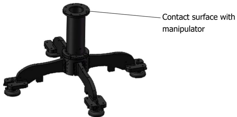
Figure 6-3 Diagram of manipulator base structure
