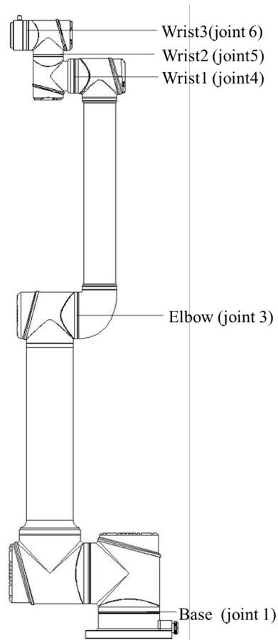
Figure 5-2 Manipulator Joints
